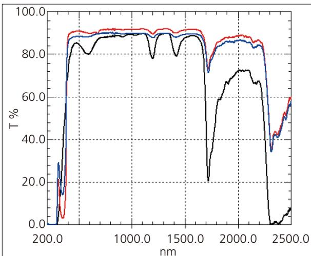
**Fig. 8 Total Transmittance (PVC)
