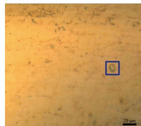
Fig. 2 Microscope Image of Contaminant (blue box size: 25 µm × 25 µm)
