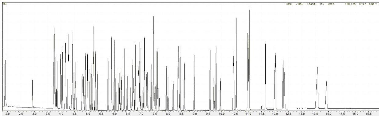
Total Ion Chromatogram of a Semi-volatile Calibration Standard. See application note #SSI-GCMS-1302, Methods 8260C and 8270D on a Single GCMS without Changing Columns, for full details.
