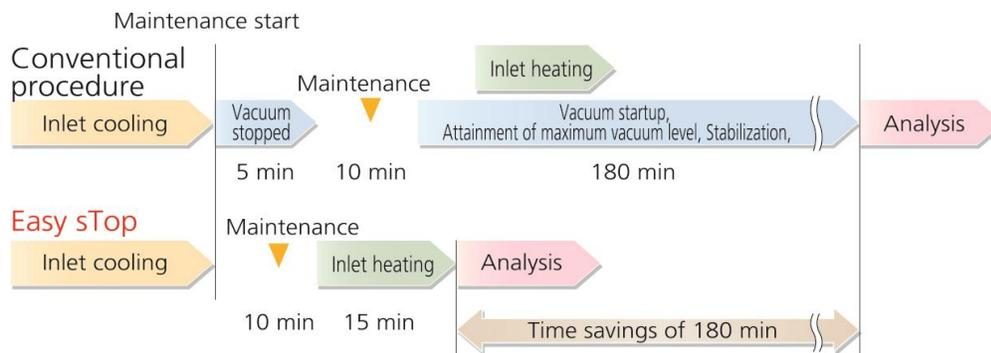
The Shimadzu GCMS-QP2010 SE reduces the maintenance time compared to other GCMS systems by efficient utilization of the following features:
