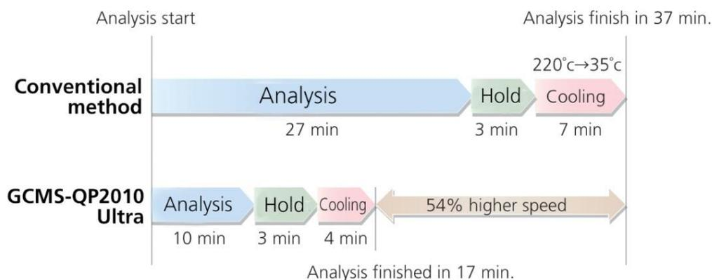
The Shimadzu GCMS-QP2010 Ultra reduces the analysis time compared to other GCMS systems by efficient utilization of the following features:
