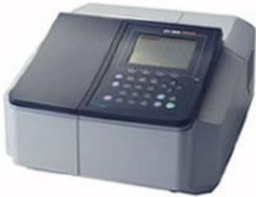
A UV-Visible spectrophotometer, such as the Shimadzu UV-1800, can be used to measure UV-254, disinfectants, or almost any of the conventional pollutants such as MBAS, cyanide, or nitrate and nitrite nitrogen. Smaller laboratories can use visible spectrophotometry methods to determine trace metals, such as iron, manganese, and chromium in drinking water samples.
