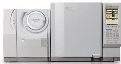
Gas Chromatography Mass Spectrometry (GCMS) combines the separation of GC with a mass selective detector that produces a fragmentation pattern specific to each analyte. This provides GC analysis with a means to obtain both qualitative and quantitative information eliminating the need for a second column confirmation. GCMS is used for the analysis of volatiles, semi-volatiles, pesticides, herbicides, and other organic contaminants in drinking water.
