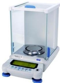
An analytical balance, such as the Shimadzu AUW-320, is used for accurate measurement of reagents for standard preparation, or for determining the mass of total dissolved solids (TDS).
