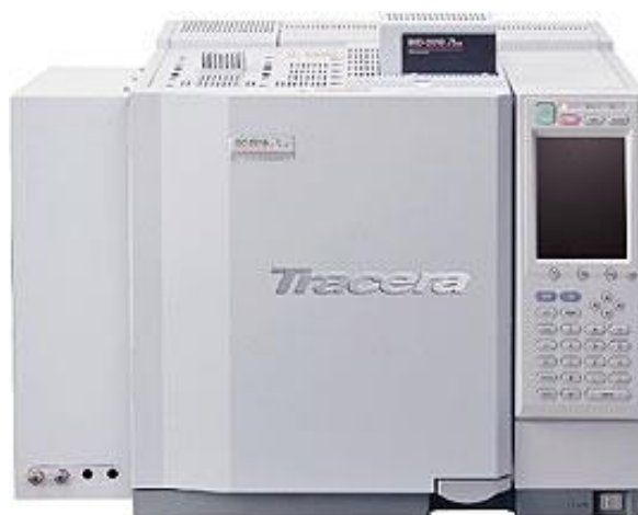
Fig. 3:Tracera(GC-2010 Plus with BID-2010 Plus) equipped with valve oven box.
